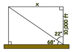
So in 10 seconds the plane traveled a distance of x feet.  $\tan(22^\circ) = x / 10000 \Rightarrow 10000^* \tan(22^\circ) = x \Rightarrow x \cong 4040$  ft
