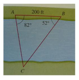
Recall the sum of the angles of a triangle must be  $180^{\circ}$ . Thus  $\angle ACB = 180 - (82+52) = 46^{\circ}$ . Let c = 200 feet Let b = distance from A to C
